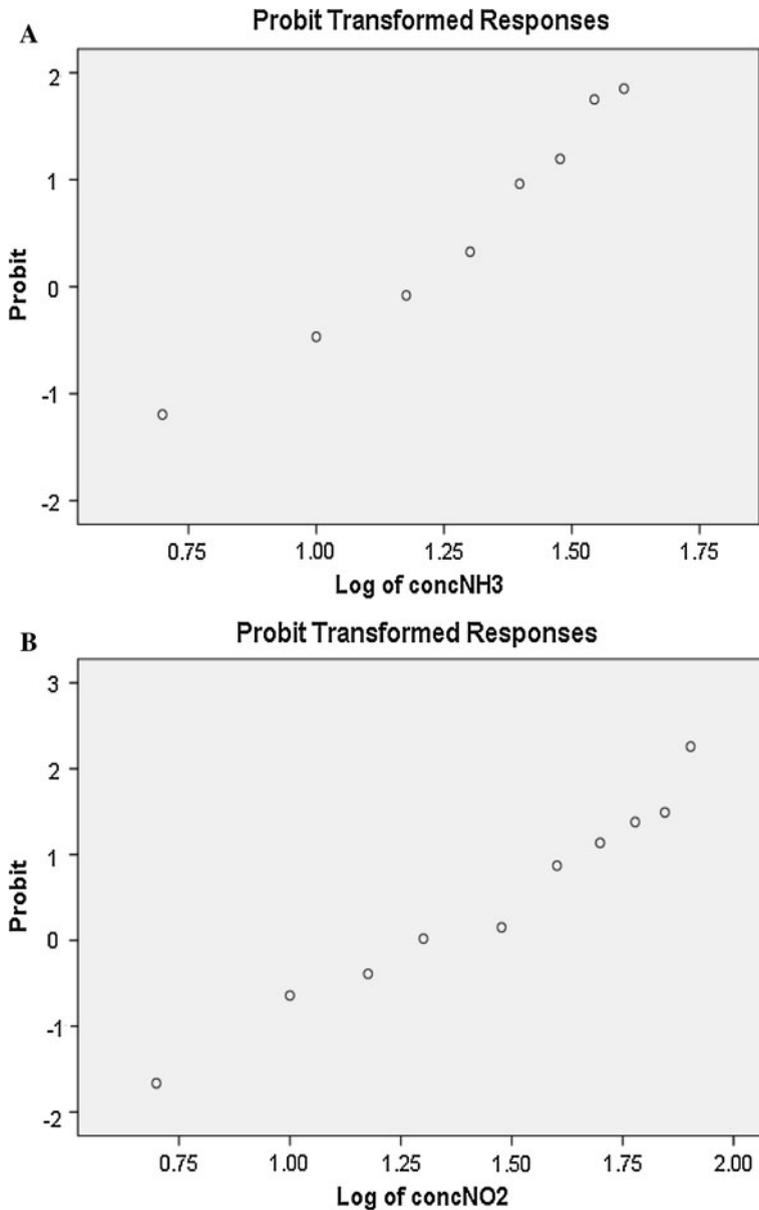
**Fig. 2** Regression plot obtained by log-10 transformation of non-ionized ammonia (a) and nitrite (b) concentrations against probit transformation of mortality percentage
